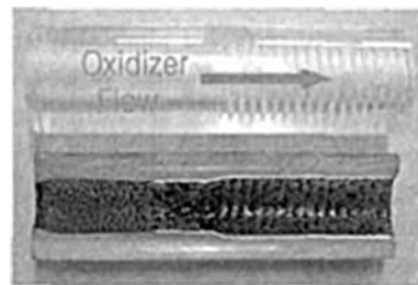
Fig. 8 Cross sectional view of solid fuel with pitch 6 before and after combustion test
